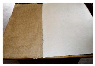
bamboo screen mesh, which is pressed, and left to drain water, leaves a bamboo imprint on the sheet. A heavy stone is placed on the pile for almost a day, to drain out the water. The sheets are then peeled off, and stuck on to mud walls of a hut, one by one. When the sheets are dry, they fall off the mud walls.
